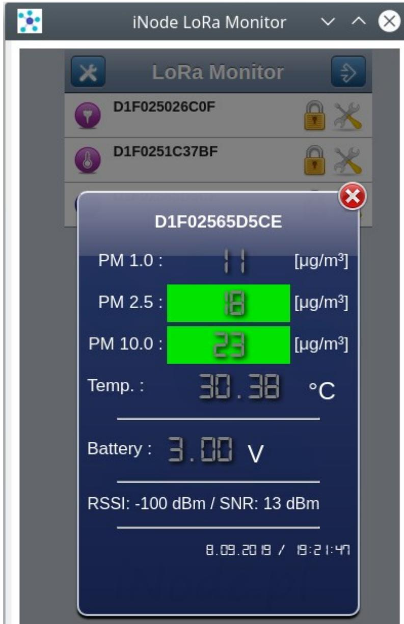
If the **iNode LoRa** device is battery powered, you can see information about the battery voltage. This voltage is measured during transmitting a broadcast frame with LoRa modulation. In idle mode and GFSK one it is higher. The minimum voltage at which **iNode LoRa** devices can work is 1.8V.
